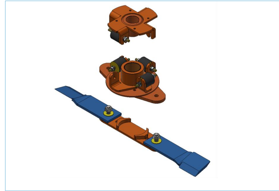
Shock absorbers for each rotor
